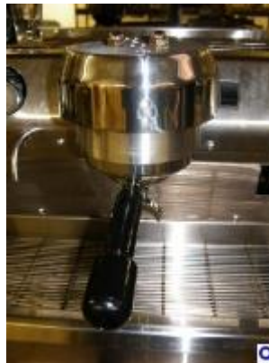
TRUEH Italia Grouphead The grouphead looks great but it is what is under the hood that counts. Pump is activated by twisting the metal cap-simple and reliable.
