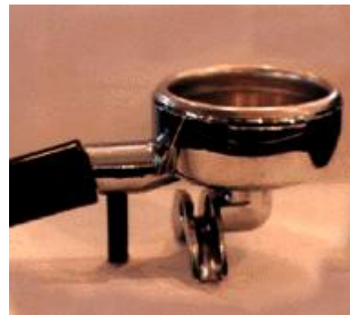
Fig. 2: The porta-filter has been modified with the addition of a post in the handle. This insures that
