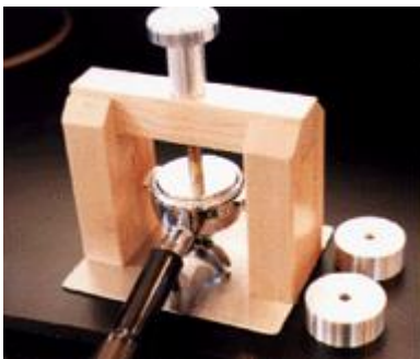
Fig. 1: The stand is made of maple, with a stainless steel base, turned aluminum handle, and packing head, with a brass connecting shaft. There are bronze bushings built into the wood for durability.
