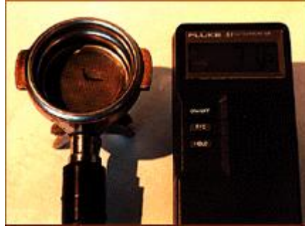
Fig. 2: To create your measurement rig simply drill a hole just large enough to admit the probe wire in the bottom of a coffee brewing basket. Run the wire up the pour spout of the porta-filter handle, through the hole you drilled in the basket and snap the basket into place.
